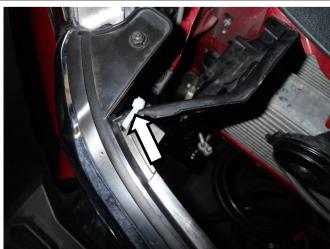
38. Cable tie the air deflector panels to the grille. (RH shown).
