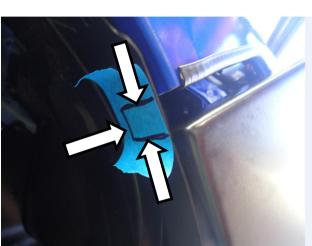
86. Push inner guard panel inside the end of the wing and behind the rear lip of the wing underpanels.
