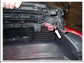
19. With grille and bumper removed, remove LH and RH headlight retaining fasteners to allow headlight to be moved forward giving access to indicator/headlight wiring.
