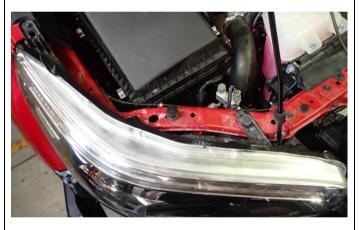
21. Re-install LH and RH headlights using fasteners retained from step 19.
