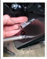
NOTE: IF USING A LARGE SIZE SOCKET, IT MAY BE NECESSARY TO PLACE THE SOCKET OVER THE FRONT BOLT BEFORE INSERTING AN EXTENSION THOUGH THE HOLE IN THE FLANGE.
