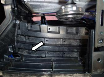
5. Remove the scrivets used to fasten the lower grille tabs to the upper crush panel. (Right hand side shown).
