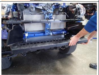
11. Remove plastic lower crush absorber from vehicle and discard.
