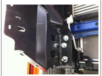
71. Adjust position of bar left/right until it's sitting central to body, then tighten all inner fasteners joining mount assembly to chassis brackets (2 x M10 and 1 x M10 OE bolts each side).
