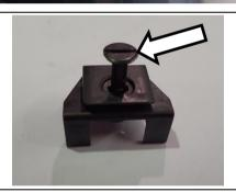
87. From the scrivet clip removed from the vehicle earlier remove the scrivet screw and set aside.
