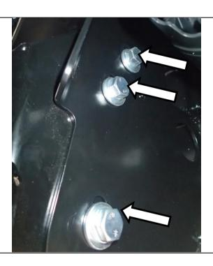
70. Loosely fasten bar to mounts using 6 x M12 x 1.75x35mm bolts, 6 x M12 spring washers, 6 x M12 flat washers (4mm thick) and 6 X M12 flange nuts.
