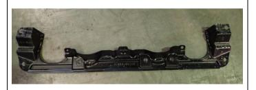
7. Remove dressing piece from underside of bumper and discard.
