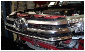
35. Re-install trimmed bumper ends and grille using retained OE fasteners.
