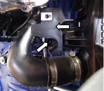
Remove M8 fastener from upper crush panel support brackets. Remove support brackets from vehicle and discard. (Right hand side shown).
