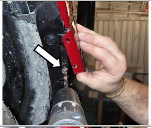
91. Using a 7mm drill bit, drill the previously drilled 3mm holes in the inner guard and bumper out to 7mm.
