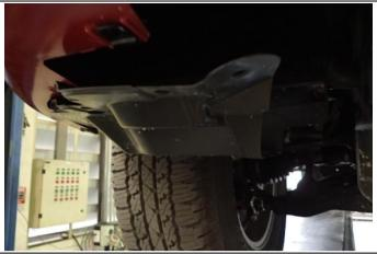
8. Ensure inner guards are unclipped from front bumper.
