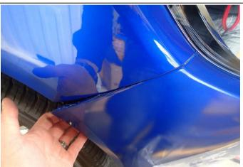
10. Remove registration plate and set aside, then carefully remove bumper from vehicle by pulling on each side of the bumper near the wheel arches and working your way towards the centre.
