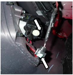
9. Disconnect fog light wiring – (Right Hand side shown).
