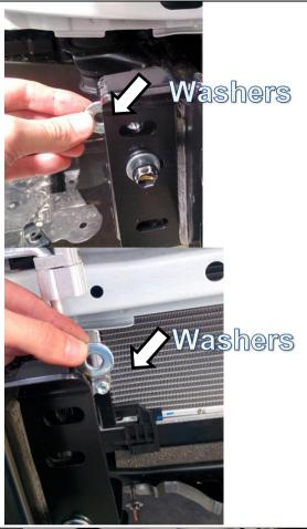
44. On both RH And LH installation it is extremely important that 1 x M10 x 25 x 3mm flat washer per hole is installed on the upper holes between the support brackets and the mount when offering the mount up to the chassis flange. The upper M10 bolts as installed in Step 47 should pass through the mount, spacer washers and the support brackets.
