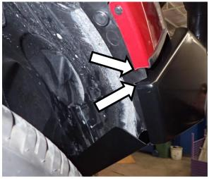
85. In line with the bottom edge of the lower bumper trim and the top edge of the bulbar wing tip use a pair of shears to cut a section approximately 20mm x 20mm from the inner guard outer edge to allow it to be pushed into the end of the wing. (RH Shown).
