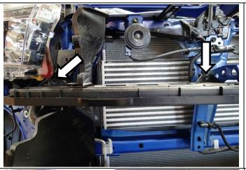
12. Remove 3 x M8 fasteners from upper crush panel. Remove crush panel from vehicle and discard.
